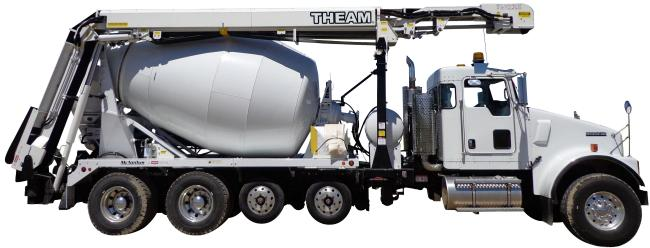
**TLS-SINGLE TELESCOPIC** MEET THE MOST POPULAR CONVEYOR IN THE LINEUP. This conveyor was introduced in the late eighties and to underscore its durability there are several original units in operation today. It has expanded reach and expanded telescoping capacity 35-52 ft. From one position you can achieve considerable placing range. This is a good conveyor choice for operations entering placing service particularly if you are servicing a single batch plant operation in a rural area.
